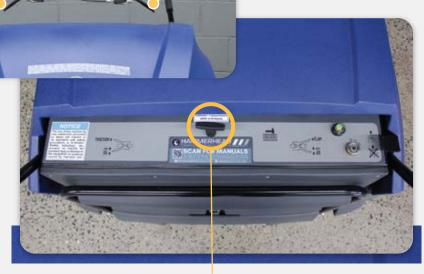
**FILTER SHAKER CONTROL** Do not "yank" on handle like starting an engine. Raise & lower swiftly to empty contents of filter into hopper.
