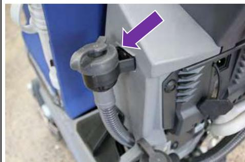
2. Check the cleanliness and sealing of the **solution filter**.
