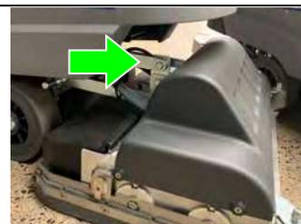
3. Adjust the pressure relief **spring** by tightening the M6 screw on the tie rod until 5-6 mm of thread remain, so as to obtain the correct pressure on the base.
