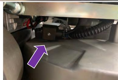
6. Check the **detergent tank drain and level hose**.
