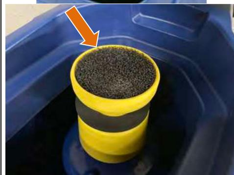
3. Check the seal between the **vacuum head** and the recovery tank.
